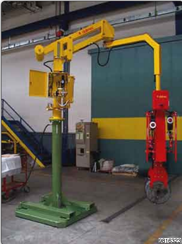
PMC type Partner manipulator, column mounted, provided with pneumatic action gripper for picking coils of wire on flanges with a pneumatic inclination of 90°.
