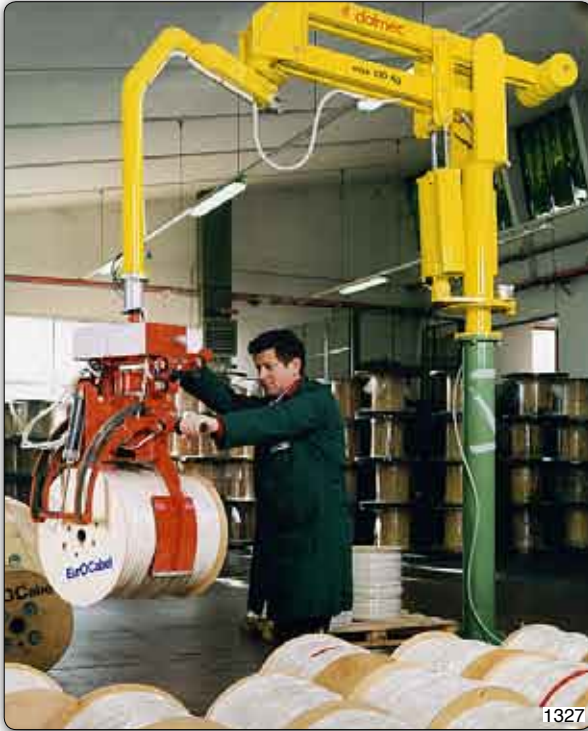
PMC type Partner manipulator, column mounted, equipped with pneumatic action tooling for picking coils of wire on the central belt, with the option of pneumatic inclination from the horizontal to the vertical.
