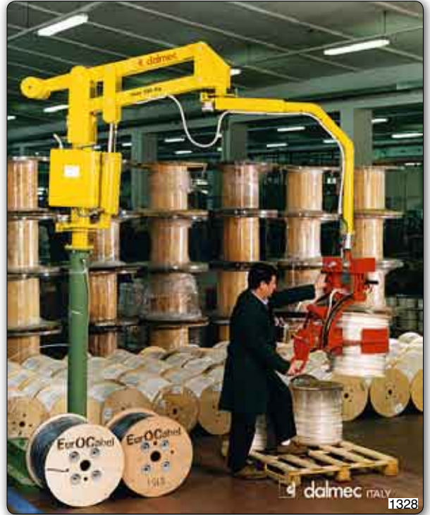
PMC type Partner manipulator, column mounted, equipped with pneumatic action tooling for picking coils of wire on the central belt, with the option of pneumatic inclination from the horizontal to the vertical.
