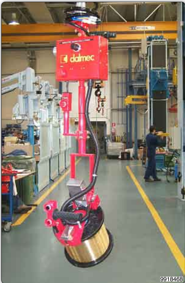
Manipulator designed to pick on the coil's flange with pneumatically actioned tooth, with manual inclination of the coil from the vertical axis to 60 degrees.
