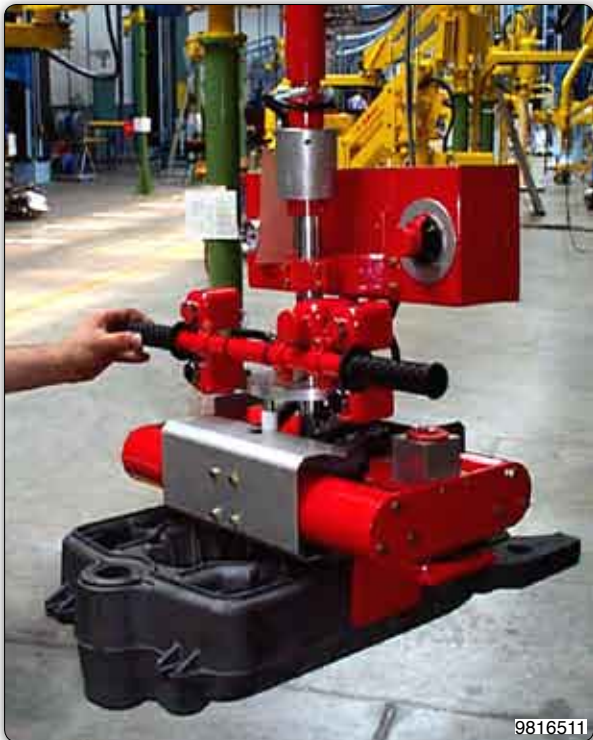
Manipulator equipped with a pneumatic gripper tooling for picking and handling parts of boilers.
