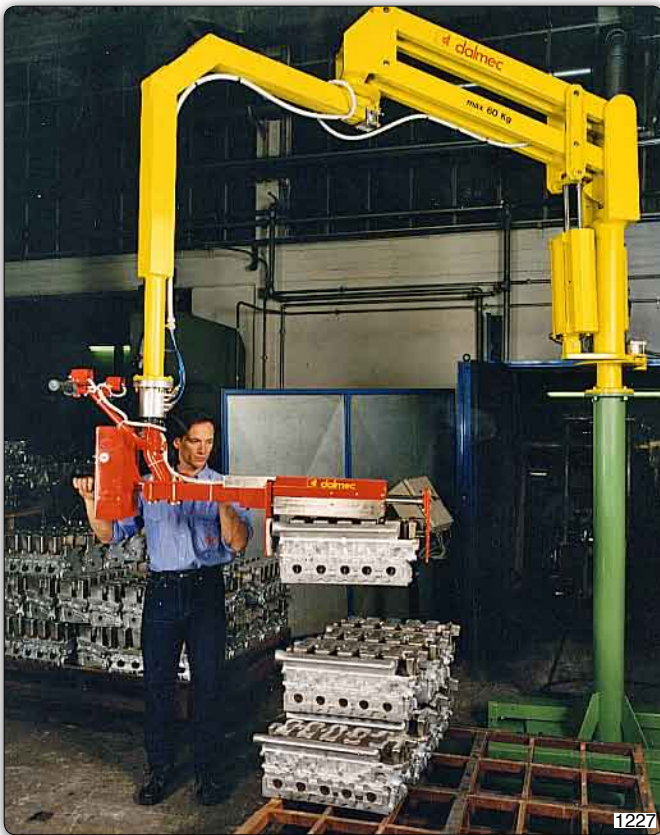
PMC type Partner manipulator, column mounted version, equipped with gripping jaws for moving aluminium cylinder heads.
