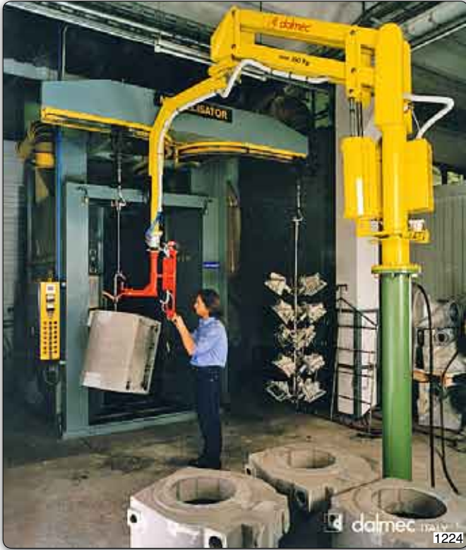
PMC type Partner manipulator, column mounted version, with special hook for handling castings.
