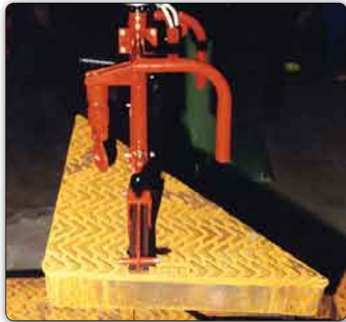
PMC type Partner manipulator, column mounted version, equipped with tooling for handling cast-iron covers.
