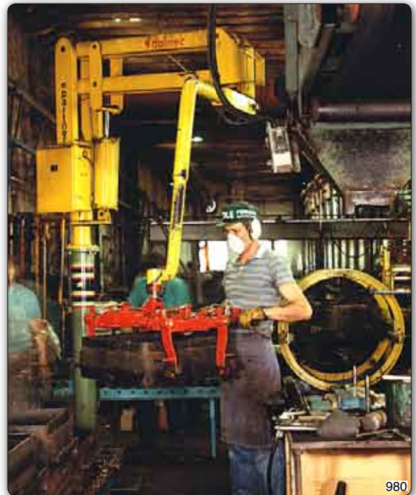
PMC type Partner manipulator, column mounted version, equipped with gripper picking system for moving cores.
