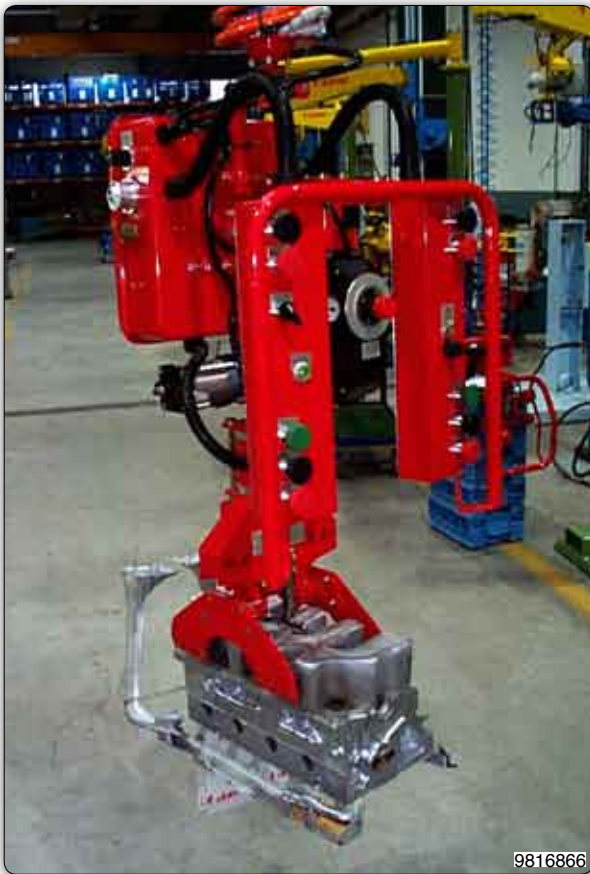
Manipulator equipped with a pneumatic gripper for picking and handling aluminium cylinder heads.
