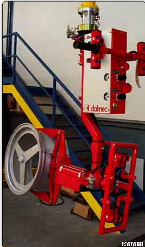
Manipulator with tooling for picking alloy rings, with manual rotation.
