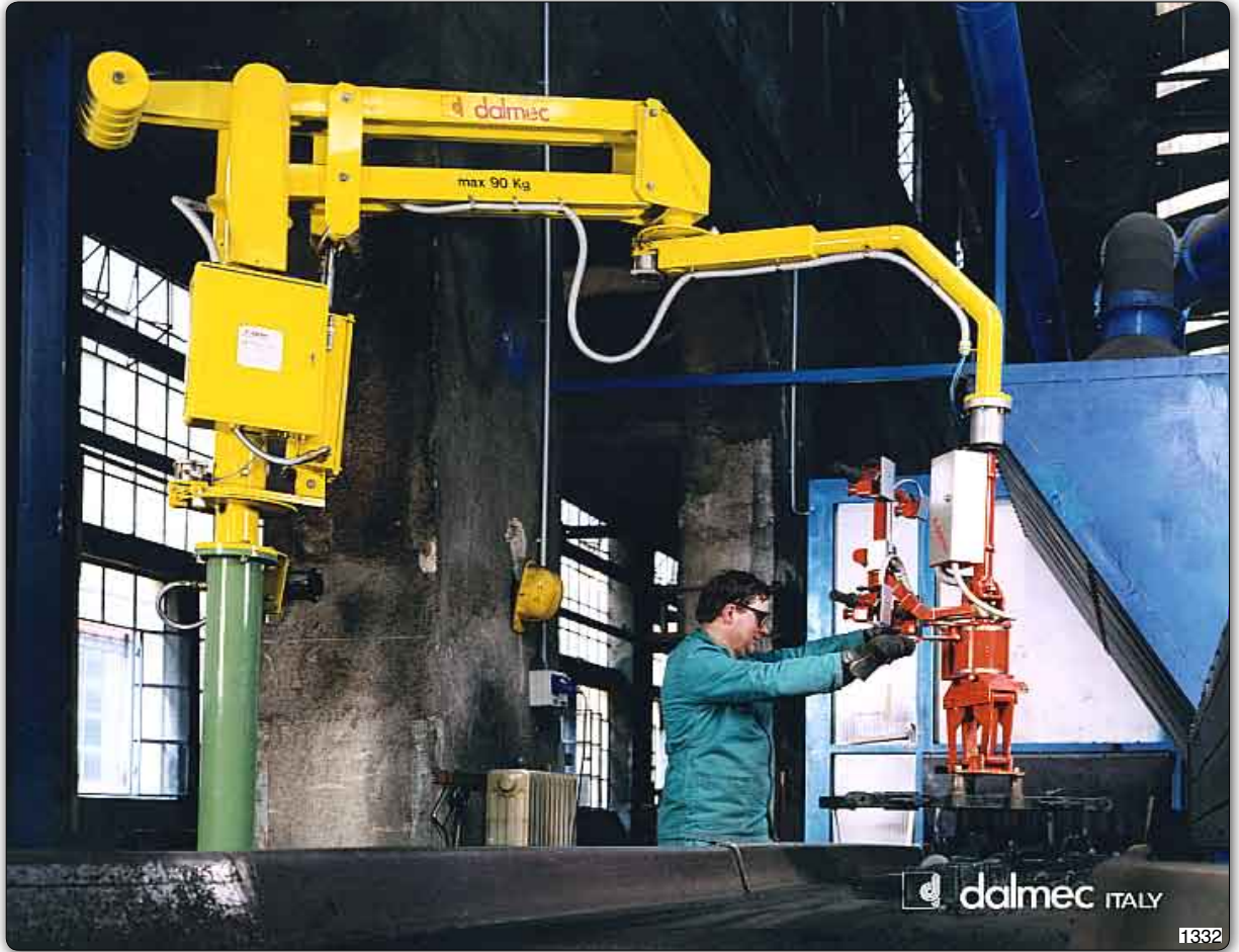
PMC type Partner manipulator, column mounted version, equipped with pneumatic gripper for castings.
