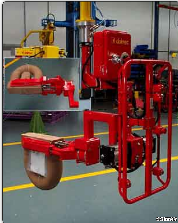
Manipulator equipped with a pneumatic gripper tooling for picking and tipping casting dies.
