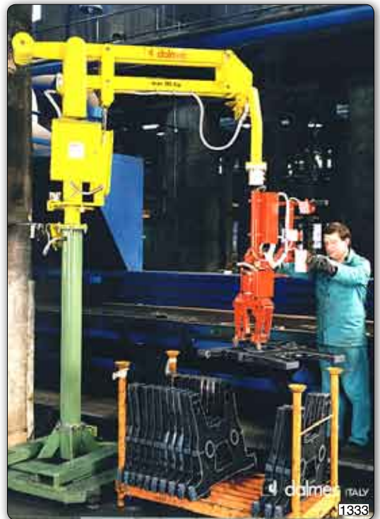
PMC type Partner manipulator, column mounted version, on portable baseplate, with pneumatic gripper for handling castings.
