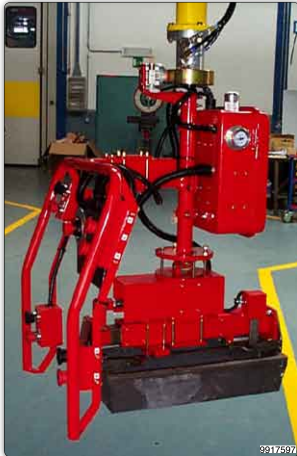
Manipulator with gripping jaws for picking and handling casting moulds.
