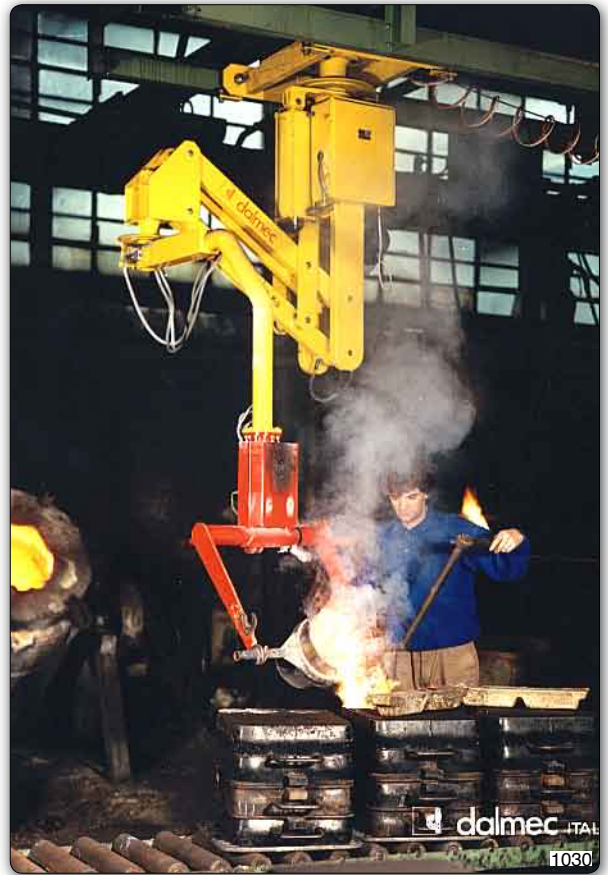
PMS type Partner manipulator, overhead trolley mounted version, fitted with fork tooling for handling ladles or crucibles.
