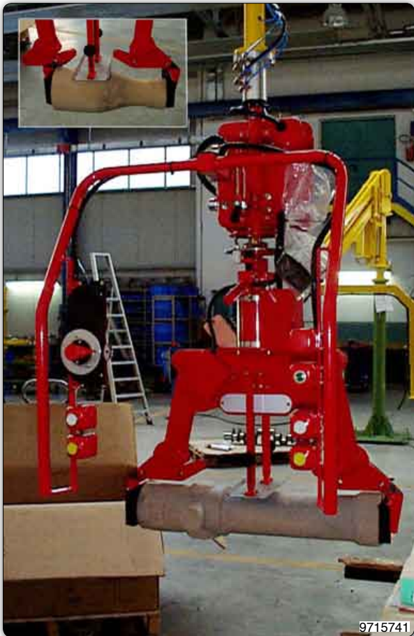
Manipulator with grippers for picking and handling cores of different dimensions.
