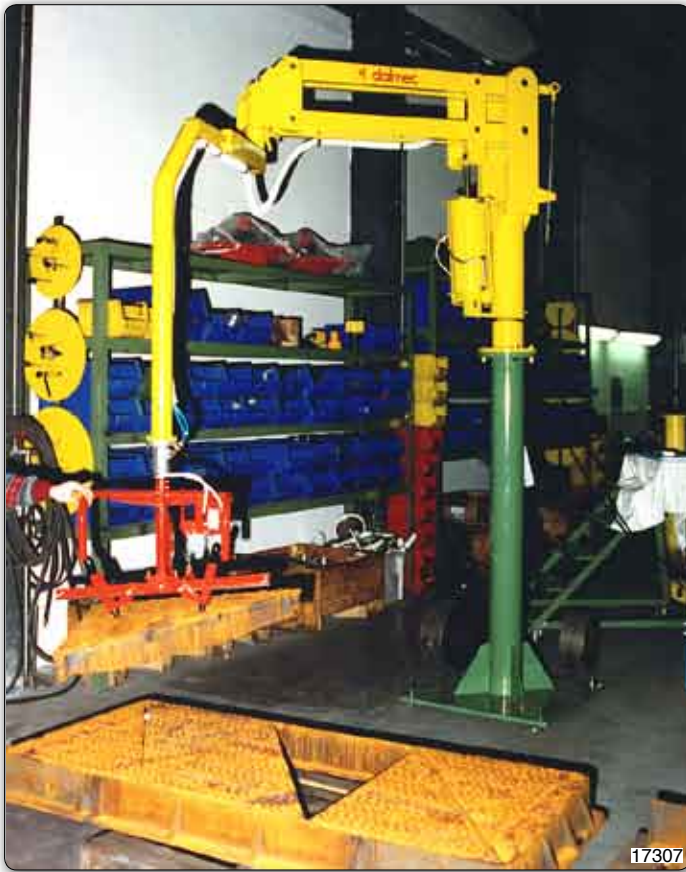
PMC type Partner manipulator, column mounted version, equipped with tooling for handling cast-iron covers.
