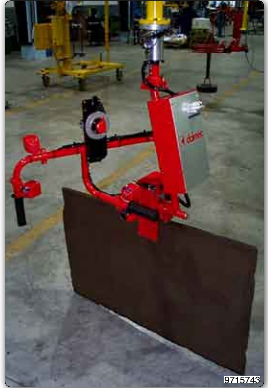
Manipulator equipped with gripper tooling for handling refractory plates.
