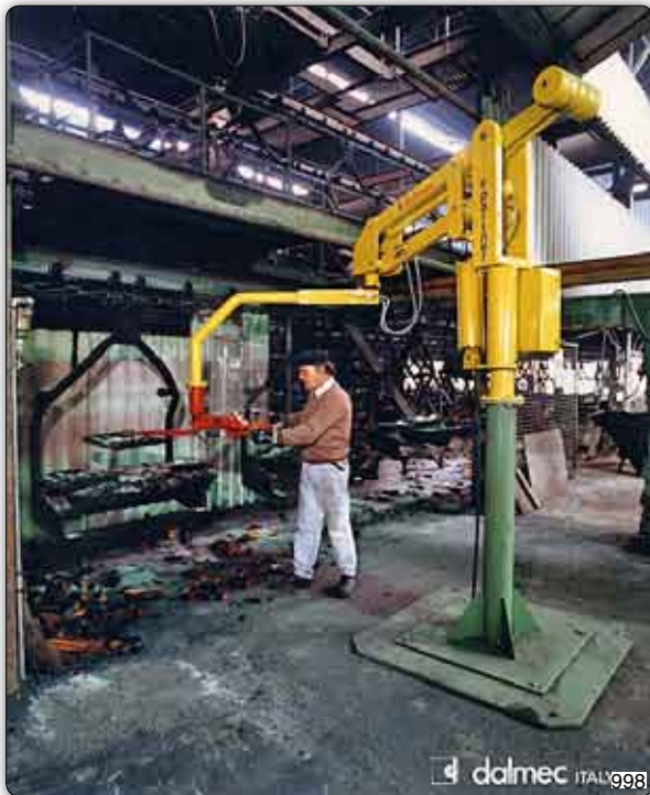
PMC type Partner manipulator, column mounted version, equipped with pneumatic gripper for handling die castings.
