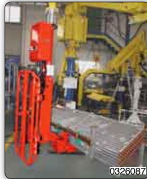
Jaws tooling for gripping and 90° pneumatic rotation of cooling coils for air-conditioners.
