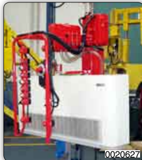
Suction cups tooling for gripping and 90° pneumatic inclination of convectors.
