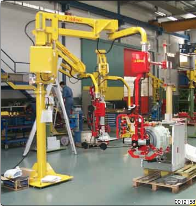
Partner PMC column mounted Manipulator, with pneumatic tooling for gripping, rotation and releasing of washing machine baskets into the frames.
