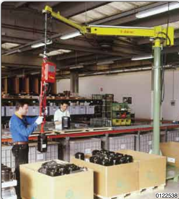
PFC type Posifil Manipulator, column mounted version, equipped with suction tooling for handling refrigerator compressors. 0122538
