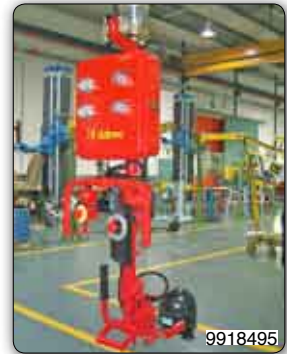
Jaws tooling for gripping and handling compressors for refrigerators.
