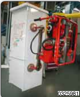
Suction cups tooling for handling and 90° pneumatic rotation of refrigerators.
