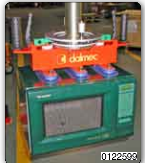
Suction cups tooling for gripping and handling microwave ovens.
