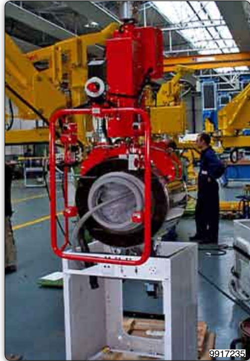
Pneumatic tooling for handling and releasing of washing machines baskets from the top surface, into the frames.
