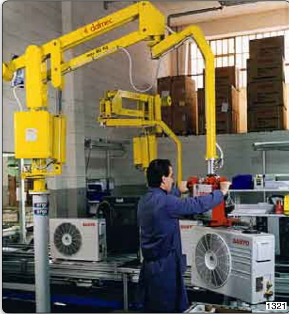
Partner PMC column mounted Manipulator equipped with suction cups tooling for handling air conditioners. 1321
