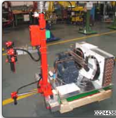
Forks tooling for gripping groups of refrigerators (compressor - panel heat exchanger). 0224438
