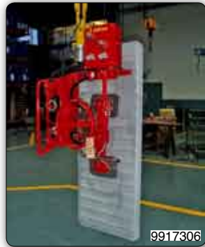
Suction cups tooling for gripping exchanger panels for cold stores.
