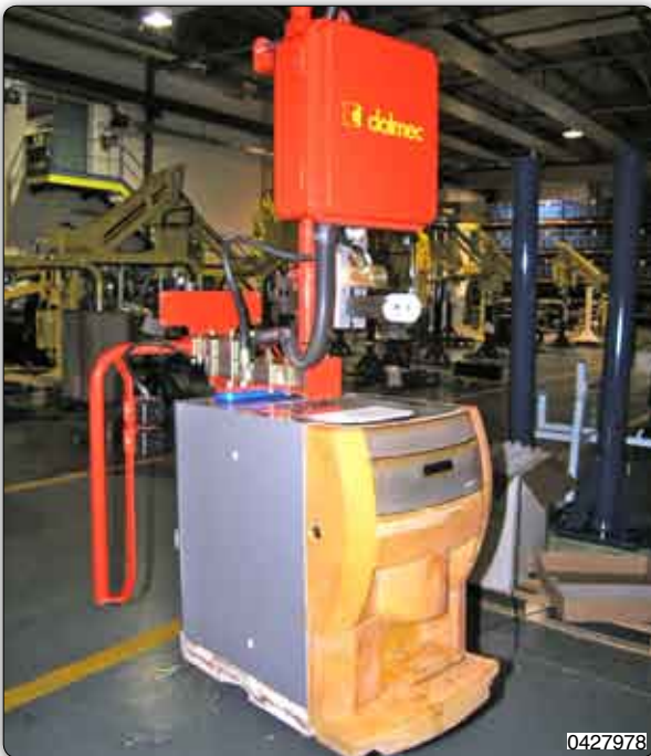
Manipulator with suction cups tooling for gripping and handling drink machines.
