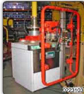
Suction cups tooling for gripping and handling electric ovens.
