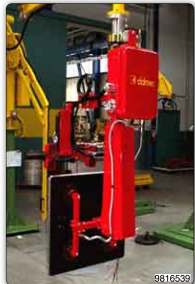
Manipulator with suction cups tooling for gripping and handling cooktops.
