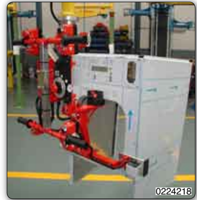
Hook tooling for handling coverings of washing machines. 0224218
