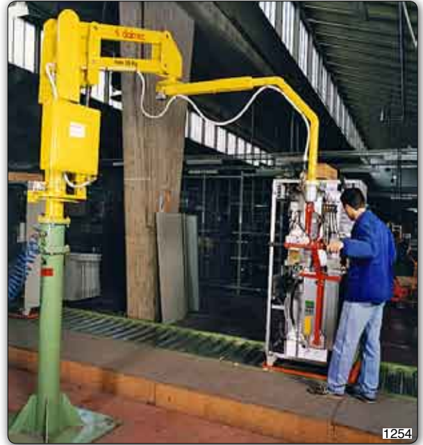
Partner PMC column mounted Manipulator with forks type tooling for handling parts of drink machines. 1254
