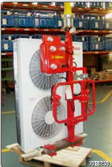
Manipulator with forks type tooling for handling air conditioners on a pallet.
