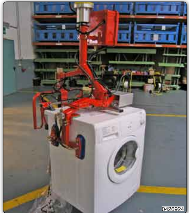
Manipulator with suction cups tooling for gripping and handling washing machines.
