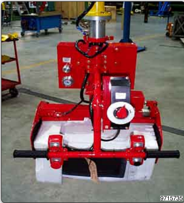
Manipulator with jaws tooling for gripping and handling microwave ovens.
