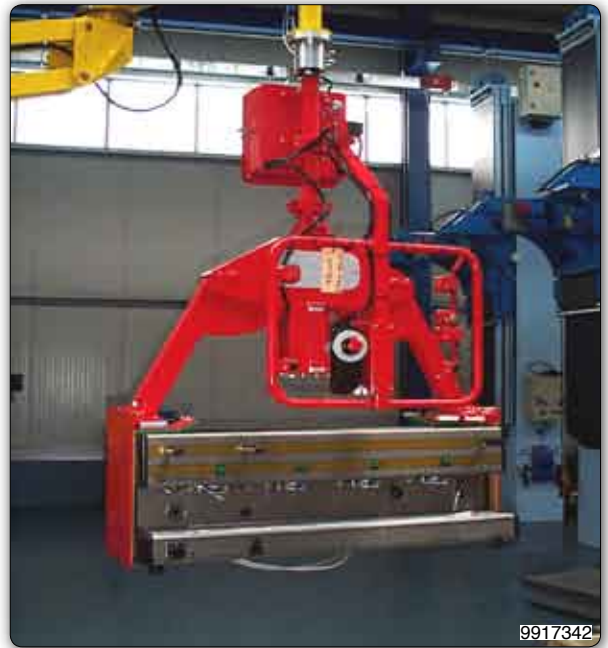
Manipulator with jaws tooling for gripping and handling coffee machines.
