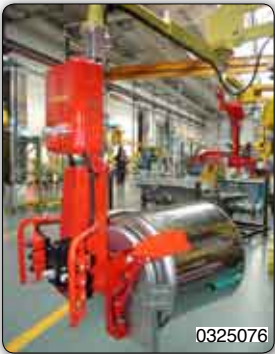
Pneumatic tooling for gripping and 90° pneumatic inclination of washing machines.
