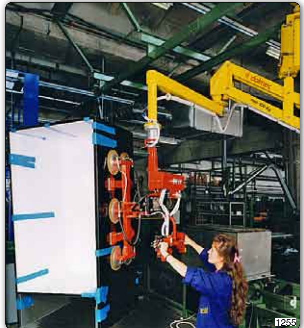
Partner PMS overhead trolley mounted, fitted with suction cups tooling for handling refrigerators coverings. 1255
