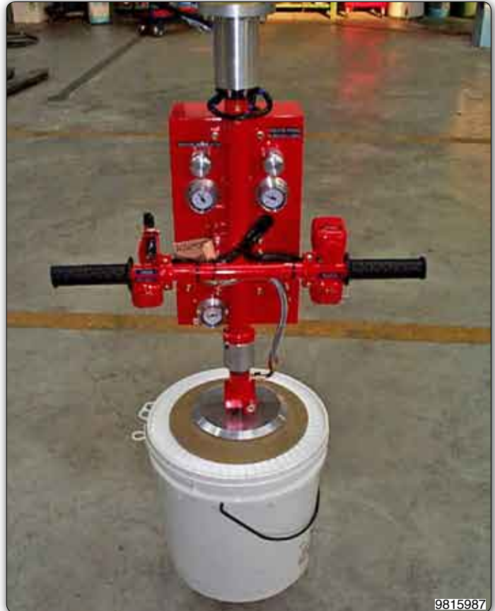
Manipulator equipped with venturi vacuum system for gripping and handling drums.
