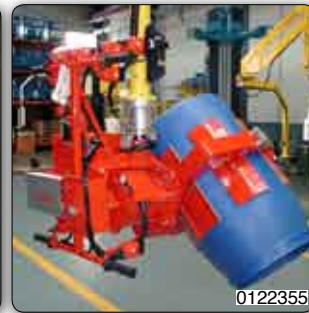
Manipulator with gripper system for picking drums on the rim with dual and low level controls.
