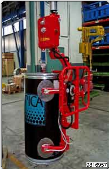
Manipulator fitted with suction cup tooling for handling drums.
