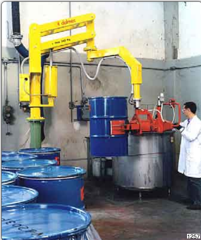
PMC type Partner manipulator, column mounted, designed for the picking and emptying of drums.
